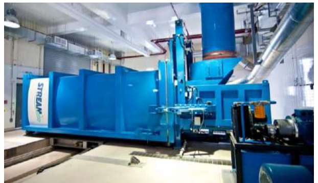
Compactor container – Automated operations, compact waste and stored in air tight container.
