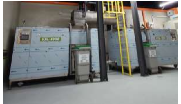
Food Waste Composter/Digester – Food waste undergoes process to be form into compostable material.
